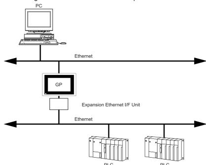
◆ When using the GP/GLC Unit's Rear Face Expansion Ethernet I/F
